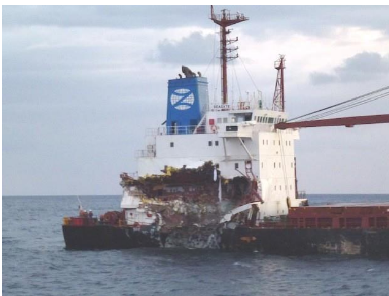
Blindsided: The M/V Seagate , severely damaged after being struck by the bow of the Timor Stream . Photo: USCG
